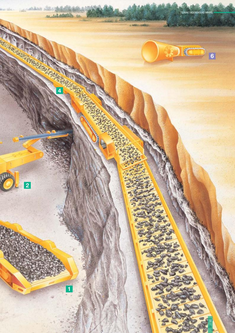
Shuttle cars are the workhorses of the underground mining system, transferring coal from the development face to the transport conveyors.
