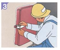
**3.** Complete installation. After the area has cooled, attach the lever, apply the gasket, and place the safety warning label in a prominent position.
