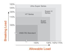
If you've had problems such as fatigue breakage of link plates, or generally poor performance, we recommend that you try the Tsubaki HT Series, Super Series, Super-H series or the Ultra Super Series, where you can dramatically increase the strength of your chain without having to make major modifications to your existing equipment.
