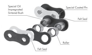
Fig. 10 Basic Construction
