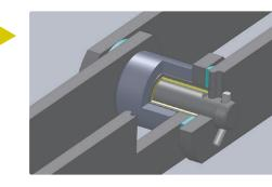
A solid lubricant is bonded between pin and bush, and an O ring is attached between the links to prevent the conveyed material from entering the link mechanism. At the same time, it retains the solid lubricant in place. This design suppresses wear between the pin and bushing (which contributes to pitch elongation), thus doubling the service life. Thanks to the solid lubricant ,bucket elevators can now feature low-noise operation with an average noise reduction of about 2dB.
