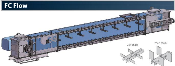
TSUBAKI FC FLOW is a continuous drag conveyor, which is appropriate for powdery or granular materials of cement, chemical and fertilizer. Materials are conveyed smoothly like water flow, along with chain running motion within a casing on a horizontal or moderate inclination layout.
