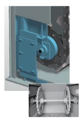
TSUBAKI Internal Take-up keeps the factory environment clean by preventing powdery materials from spilling from the casings. This take-up utilizes the weight of the tail mechanism to provide automatic tensioning. The take-up components are housed in the tail casing and are completely enclosed, however they are easily accessible for inspection and maintenance.
