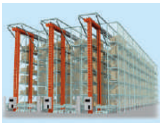
Automated stacker crane
