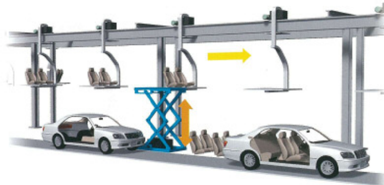
Lifting weight : 200kg Stroke : 4,000mm Lift speed : 30m/min
